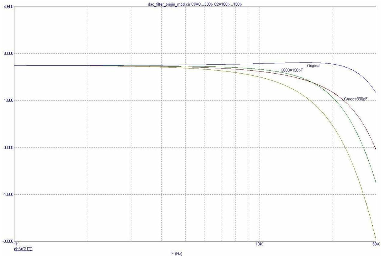
In this first graph we can notice the following: the comparison between the T.Loesch's original filter, in TnT-Audio articles (with 150pF instead of 100pF) and the filter elaborated by M. Penasa with the suggested differential filter capacitor (330pF).
