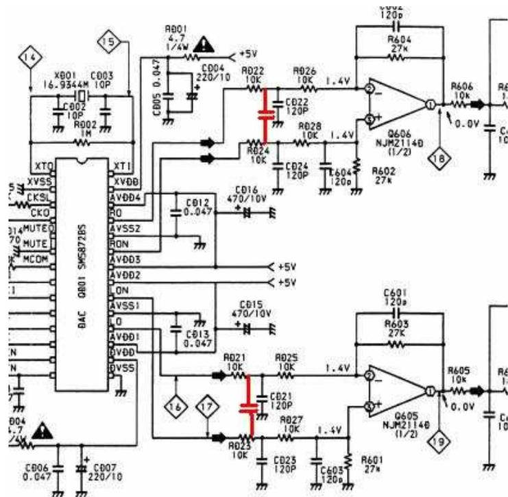
You will notice the presence of the new parallel capacitor at the DAC's outputs, below the first Rs of the filter.
