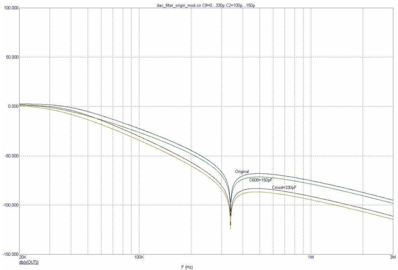
Here we show the same comparison in the area of influence of the PWM (20Khz to 3Mhz) You will notice that the version with 330pF follows a much stronger cleaning action of the new, changed, filter starting from 50khz if compared to the T.L. original version . It becomes more efficient of about 20dB in the critical zone of the PWM (about 350khz where
